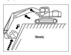
It is easy to control the boom RAISE, so the cutting edge does not deviate from the boulders
