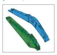
The revolving frame, centre frame and undercarriage are designed by using advanced three dimensional CAD and FEM analysis technology.
