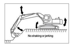
During simultaneous operations, there is no change in the work equipment speed caused by change in load. Thus, there is minimal chassis vibration.
