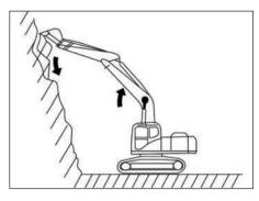
Even without operating the lever to the maximum position, maximum digging power can be obtained, making it possible to carry out slow control.
