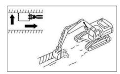
Lateral power pushing is powerful, allowing digging operation to be carried out efficiently.
