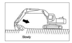
During simultaneous operations, the work equipment moves slowly at maximum power, without being influenced by the other actuators, so it is easy to fully load the bucket.
